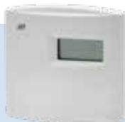
The new **KLH 100-5V-PT 1000** and **KLH 100-NTC 10** versions of humidity transmitters/controllers have passive Pt1000 or NTC 10 sensors, and the 5V-version has 0...5 V outputs. [Page 33](#)
