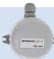
**PEL-USK** is an **outdoor protective cover for pressure hose**, especially for when you need to measure the difference in pressure inside and outside of a building. It softens, for example, pressure shocks caused by the wind and protects the hose from other environmental influences. [Page 30](#)
