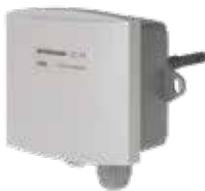
Our new **HDK-NTC 10** version of CO<sub>2</sub> transmitter/controller has a passive NTC 10 sensor for measuring and controlling CO<sub>2</sub>, temperature and humidity in ventilation ducts. [Page 37](#)
